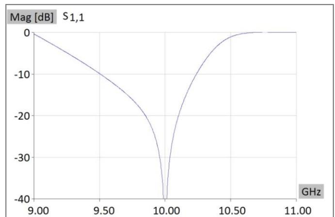
Figure 2. Parameter s11 for circuit shown in Figure 1.
