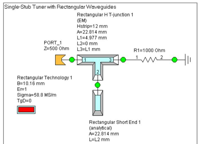
Figure 1. Single-stub tuner with rectangular waveguides
