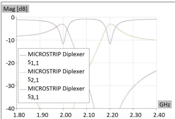
Figure 4. S parameters for network shown in Figure 3.
