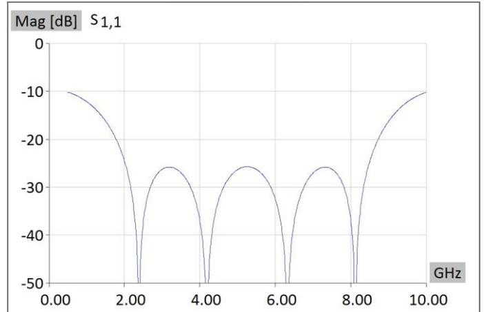
Figure 6. Parameter  $s_{11}$  for network shown in Figure 5
