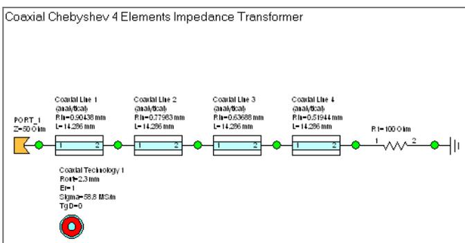
Figure 5. Coaxial Chebyshev impedance transformer
