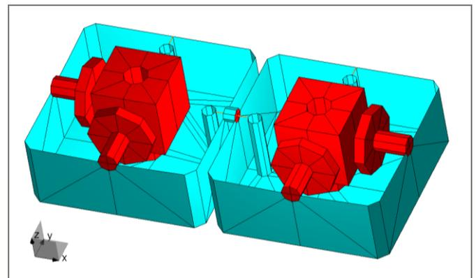
Figure 4. Interior of dielectric resonator filter.
