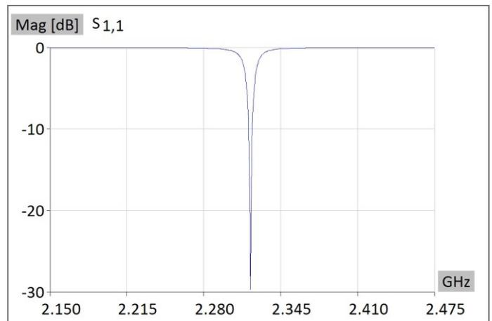
Figure 9. Return loss in frequency band around resonance.
