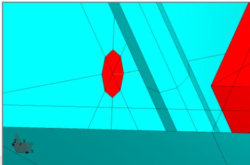
Figure 7. “Goal-post” coupling between the cavities.
