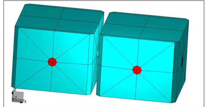
Figure 2. Layout of dielectric resonator filter.
