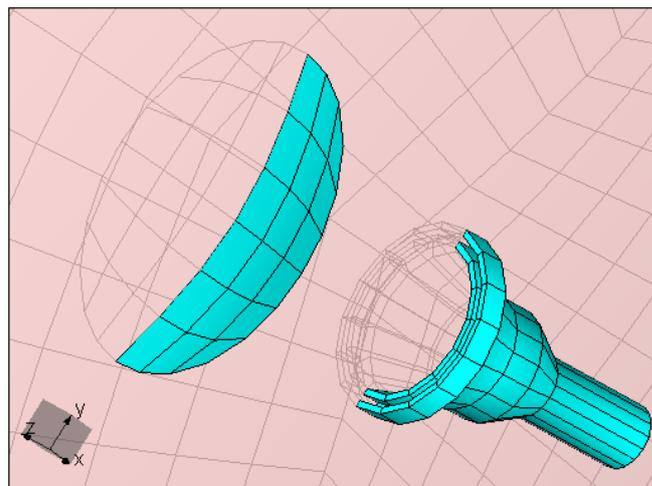
Figure 2. Cassegrain primary reflector. Half antenna model
