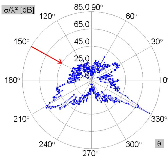
Figure 2. Radiation pattern, incident plane, at 4 GHz
