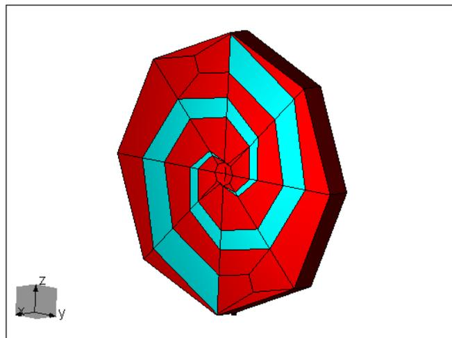
Figure 2. Spiral antenna printed on dielectric
