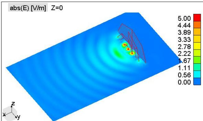
**Figure 5. Near field of spiral antenna**
