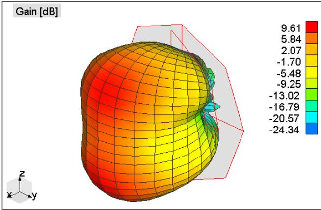
**Figure 3. Radiation pattern of spiral antenna immersed in air**
