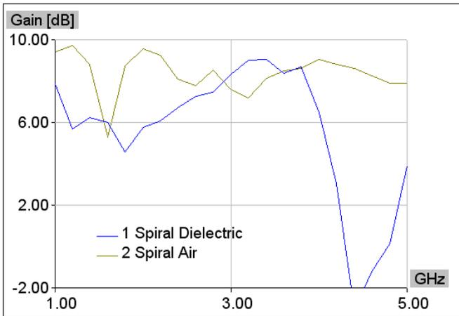
**Figure 4. Overlaid gains for main radiation direction**
