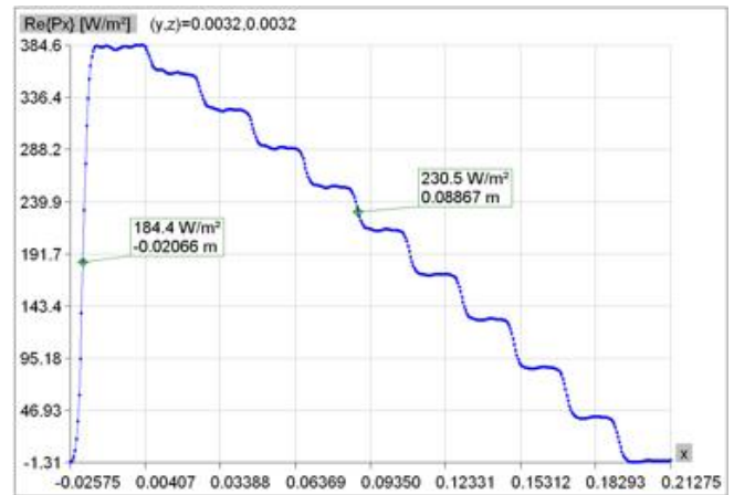
Fig.6. Real part of the Poynting vector longitudinal component along the axis of the waveguide (array)
